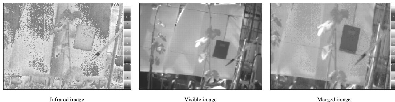
Figure 6 Overlapping of visible and thermal images to identify accurately the plant leaves
