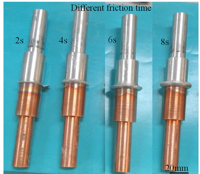
Fig. 1. Macro structures of the welds at different parameters.
