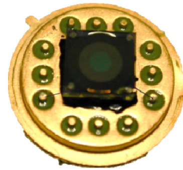
Figure 16. \mu FPF for the visible range mounted on a TO-8 header to be used in a handheld hyperspectral imager (taken from Ref. 60 ).
