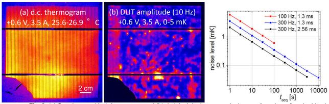
Fig. 3. (a) Steady-state (d.c.) thermogram and (b) dark lock-in thermography image of a solar cell under identic conditions, (c) measured amplitude noise levels of the InfraTec PV-LIT system.
