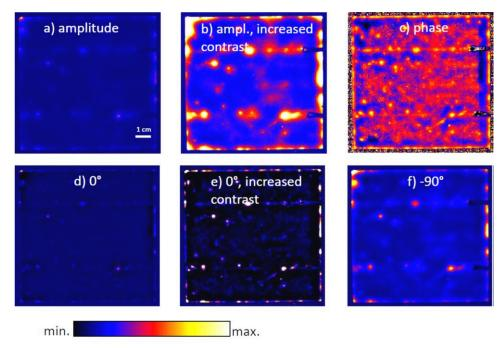
Fig. 1. Different ways to display LIT results of a solar cell, see text.
