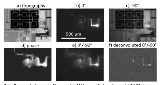
**Fig. 8.** (a) Topography image, (b) 0° image, (c) -90° image, (d) phase image, (e) 0°/-90° image, and (f) spatially deconvoluted 0°/-90° image of a region in a bare IC.
