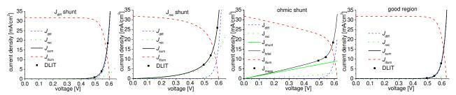
**Fig. 6.** Thermally measured dark and illuminated local I-V characteristics of different positions in a solar cell (J<sub>diff</sub> shunt, J<sub>rec</sub> shunt, ohmic shunt, and a good region).
