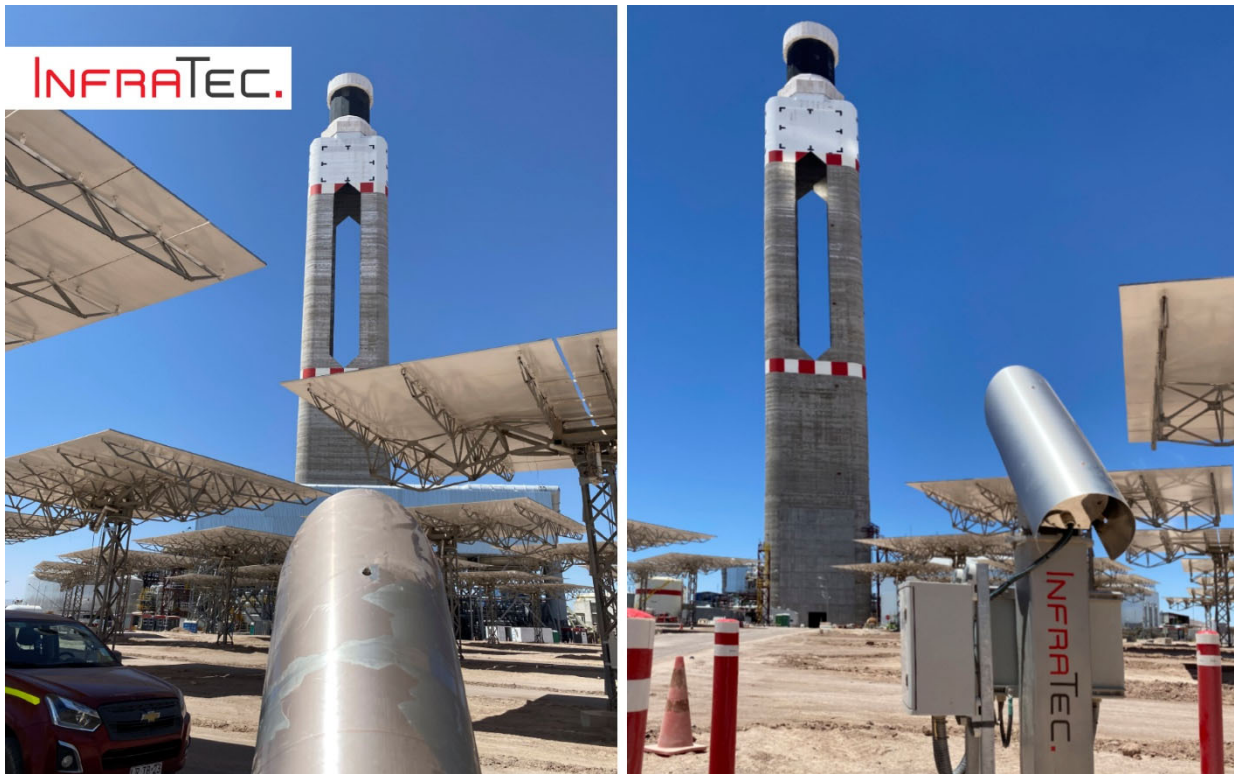
Fig. 1: InfraTec infrared camera: between the mirrors of the solar field, around the solar tower in the Atacama Desert, aligned with the tower's receiver.
