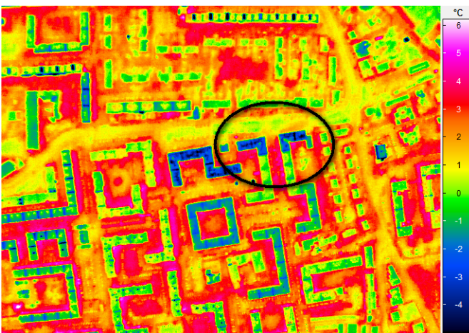
Fig. 9: 75cm GSD Thermal image. Different sections of the marked buildings show a very different roof-temperature.
