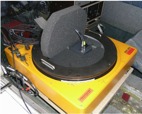
Fig. 8: DigiTHERM with thermal insulation mounted in a GSM3000 mount.
