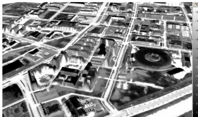
Fig. 13. 3D model from combination of DSM and True Orthoimage
