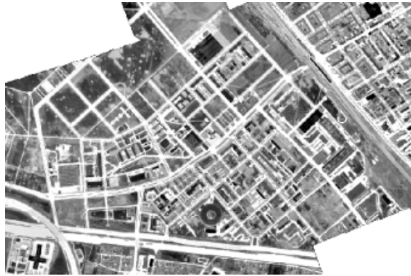
Fig. 11. Thermal orthoimage derived from ImageIR 8300 data
