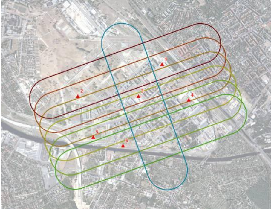
Fig. 9. Flight planning showing the extent of the image stripes (multicolor) and the position of the heat-emitting ground control points (red triangles)
