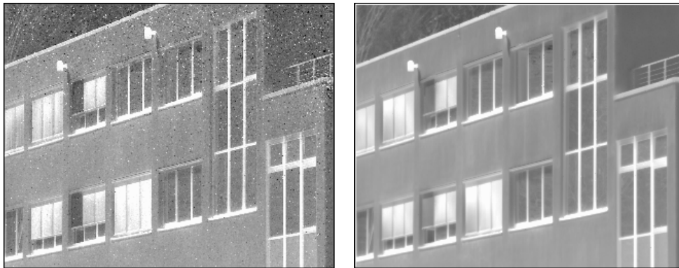
Fig. 5. Thermal images of an LWIR MCT camera after cooldown, before (left) and after (right) an internal NUC
