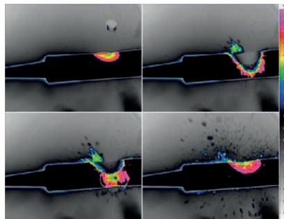
Due to the binning technology, infrared cameras have two speed modes – the standard mode and the high-speed mode, in which the frame rate increases more than three times. The field of view remains constant in both modes, so the scene captured by the camera does not change. In high-speed mode, the thermal resolution also increases by a factor of two. So temperature changes can be recorded and analyzed very fast.
