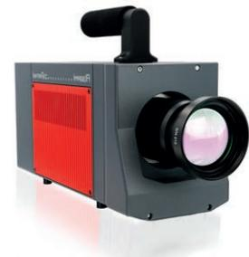
The multispectral feature makes it possible to record sequences with constantly changing spectral filters. Images are recorded synchronously with a rapidly rotating filter wheel equipped with the filters. It may be possible to switch between up to seven filters, depending on the version. Due to this multispectral measurement can be optimized to suit the measuring task if the preset ranges are unsuitable.
