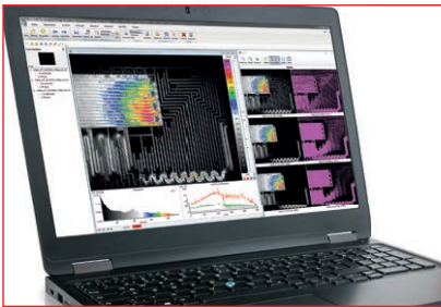
Analysis of an electronic component by lock-in thermography with IRBIS® 3 active software
