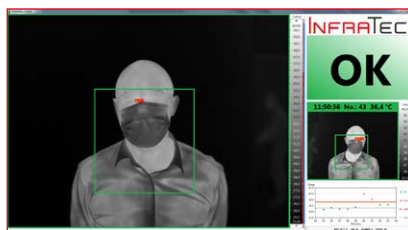
As soon as the test person enters the marked area (green field in the center of the image), the measurement starts
