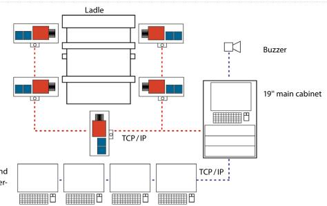
Parameterisation, supervision, operation, display, evaluation and playback on standard PC at different sites (user-level dependent)
