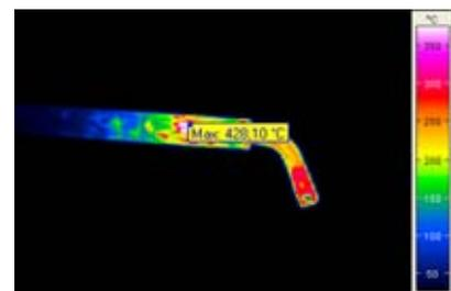
Fig. 126: Soldering iron, in focus (maximum temperature: 428 °C)
