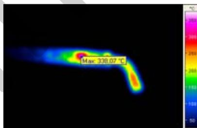
Fig. 125: Soldering iron, focused better (maximum temperature: 338 °C)
