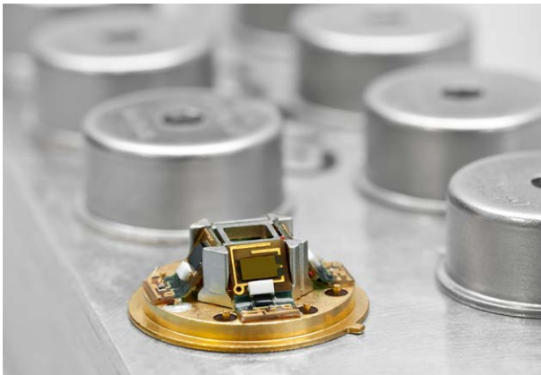
In quad channel detectors InfraTec uses four-sided micro-pyramids to split the infrared radiation.
