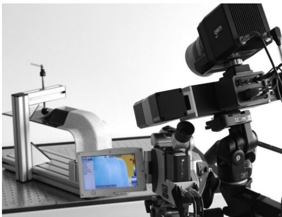
Fig. 6 ARAMIS testing of mechanical components
