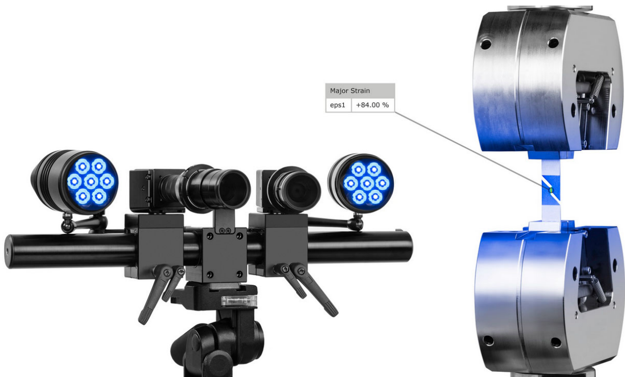
Fig. 1 ARAMIS system from GOM
