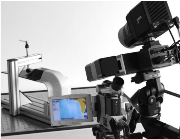
Fig. 6 ARAMIS testing of mechanical components
