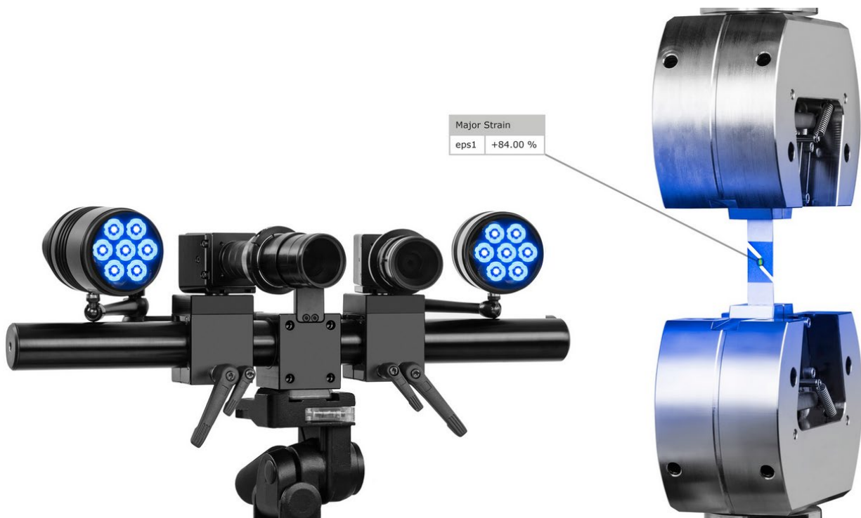
Fig. 1 ARAMIS system from GOM
