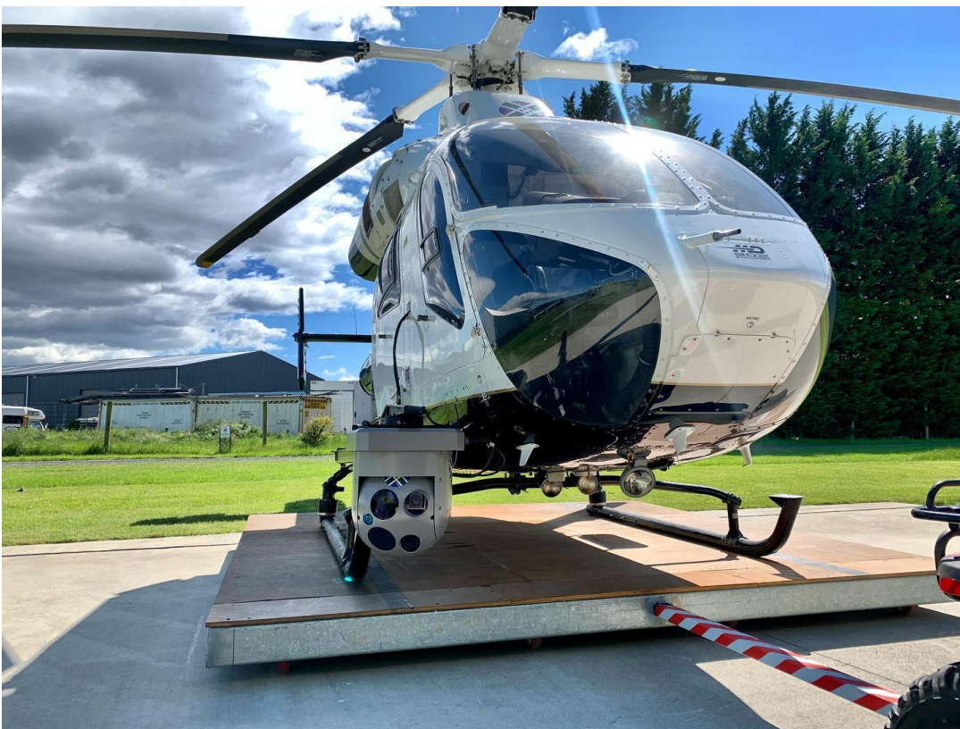
Fig. 4: Bell 206-1 LongRanger with GIMBAL system including VarioCAM® HD head 800
