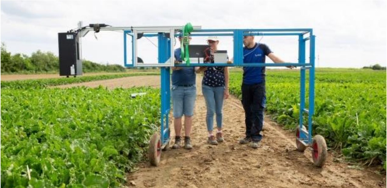
Fig. 1: The measurement set-up for determining the leaf temperature with infrared camera and monitor.
