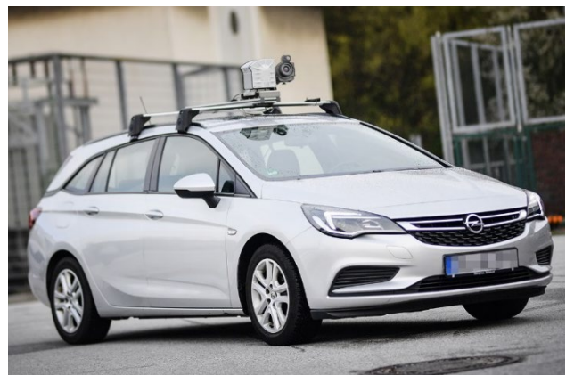
Fig. 4 Since 2017, Netze Duisburg GmbH has been using an utility vehicle equipped with an infrared camera.
