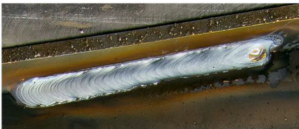
e) Colour image of a defect-free weld
