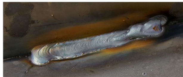
f) Colour image of a defective weld
