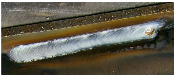
e) Colour image of a defect-free weld
