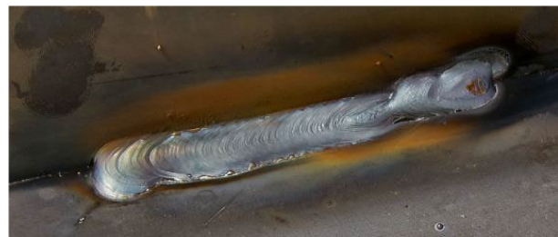
f) Colour image of a defective weld
