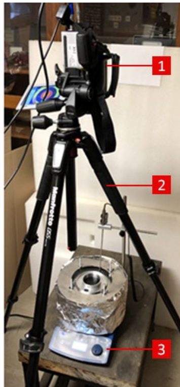
Fig. 1 The test setup should ensure, firstly that the sample is heated evenly by the surrounding metal block, and secondly, that the infrared camera captures the sample surface at a vertical angle. 1 – Infrared camera VarioCAM® HD research 800 2 – Tripod 3 – Heat source (tempered silicone oil bath with hot plate) 4 – Epoxy sample 5 – Aluminium cavity 6 – Aluminium heat accumulator
