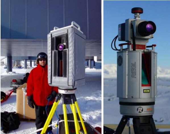
VarioCAM® HD 880 mounted on top of the RIEGL LIDAR.
