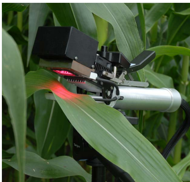
Close-up of temperature-controlled leaf cuvette and artificial light source
