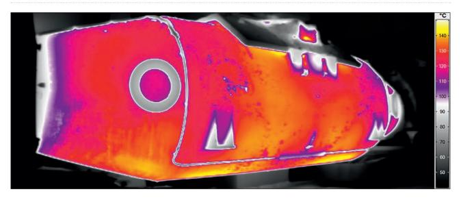
The Torpedo Hot Spot Detection (THSD) system uses Infrared (IR) technology to monitor the temperature of the torpedo steel structure. Two thermography cameras observe the torpedo cars while they are moved to the steel shop. The temperature measurements are made fully automatically without the need of any manual interaction.
