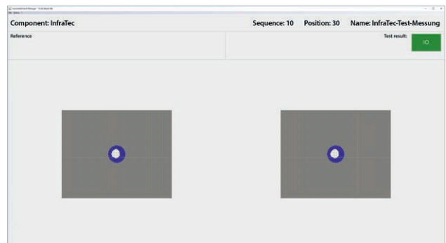
Fully automatic testing of resistance welding spots
