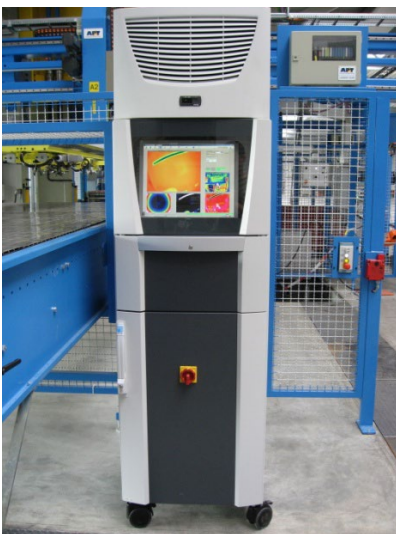
Fig. 1 Control- and evaluation unit, used to operate the press camera and to transmit evaluations to the press control
