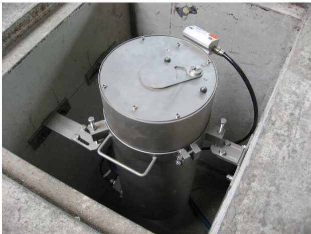
Fig. 3 Stainless steel housing with pneumatically power hatch to protect the measuring instruments, converter and sensorscomponents
