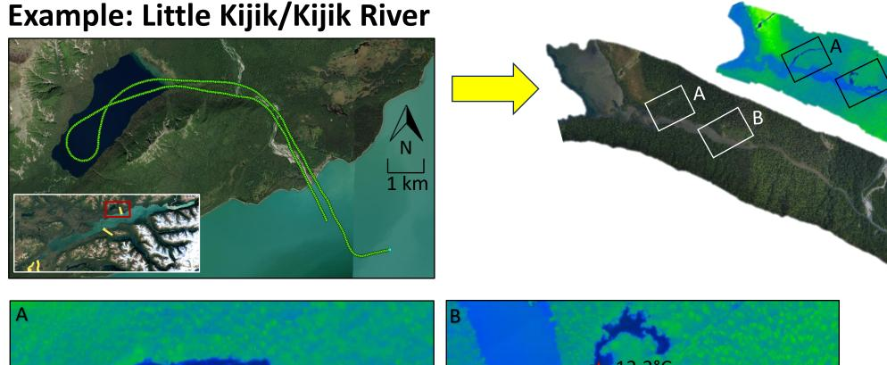
produced. From the thermal orthomosaic (scaled from 0-30°C), cold water refugia can be identified (bottom A/B).
