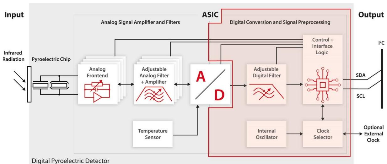
The ADC provides a 16 bits wide data word for each of the 5 channels (four sensor channels and one temperature channel) at a maximum sampling rate of 1 kHz. The signal chain inside the digital section is illustrated in the graph below.
