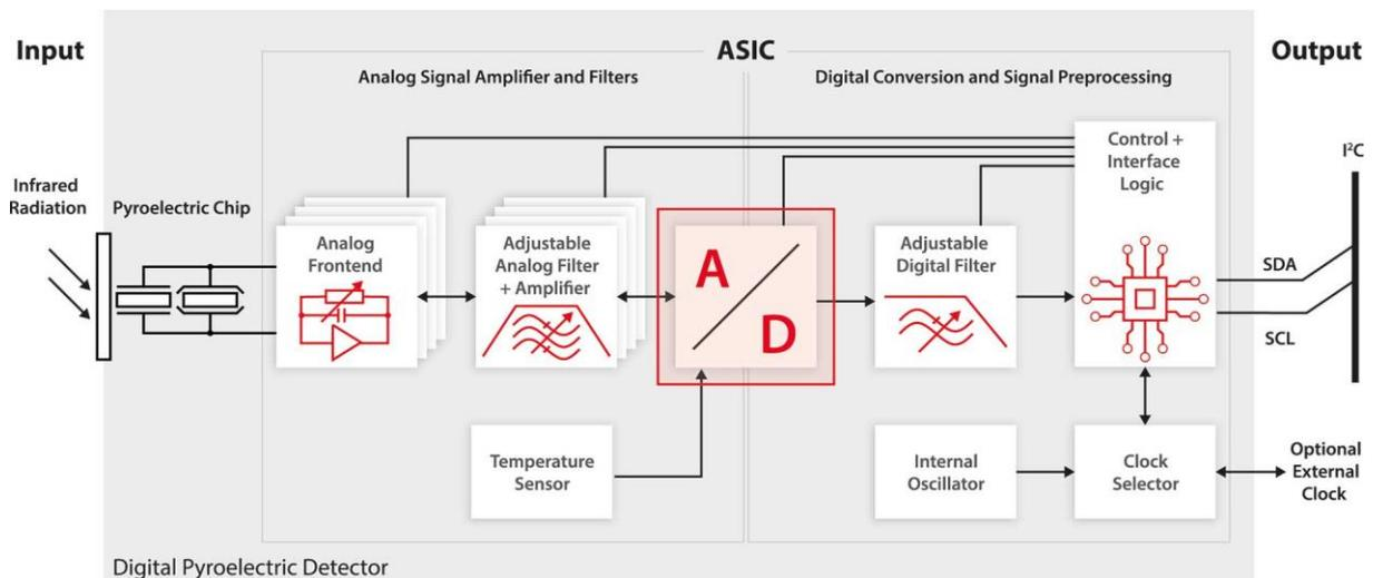
Figure 1: Schematic working principle of ASIC
