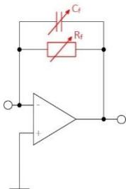
Figure 2: Analog front-end with transimpedance amplifier
