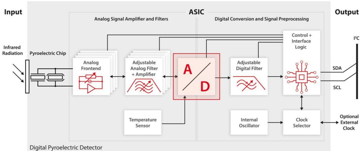
The next step after the analog section is the analog-to-digital conversion. The analog-to-digital converter (ADC) has a resolution of 16 bits, ensuring that the introduced quantization error remains significantly below the noise density of the analog front-end. Consequently, the final signal-to-noise ratio (SNR) of the system is determined by the performance of the analog front-end and is not limited by the capabilities of the ADC.
