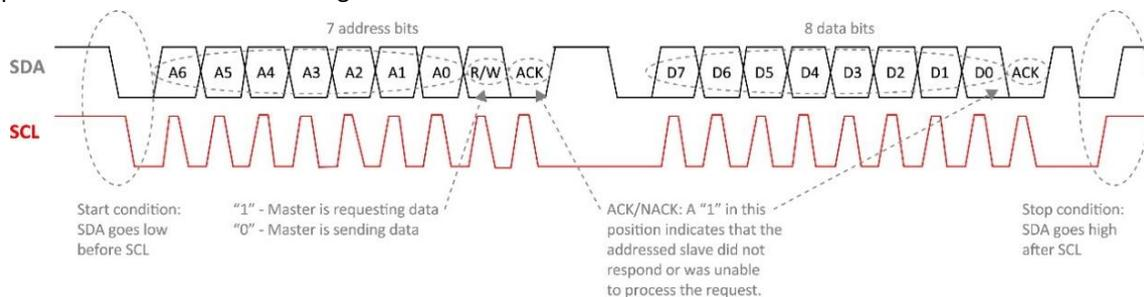
Figure 4: Typical I<sup>2</sup>C frame
