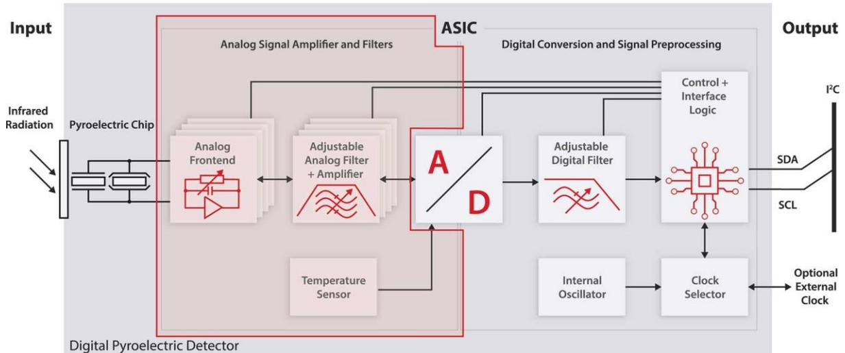
Changes in the incoming IR-radiation lead to temperature changes of the pyroelectric chip which consequently result in a small electric current in the range of a few picoamps. Because of the high output impedance of the pyroelectric material the signal cannot be used directly for evaluation purposes. The analog front-end contains the required signal processing in form of a transimpedance amplifier.
