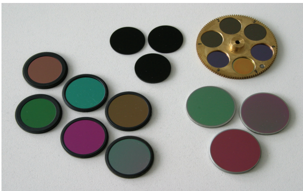
Fig. 4: Spectral filters for thermographic cameras
