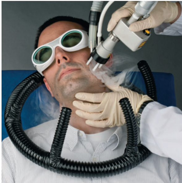
Figure 3. Clinical treatment setting simulating plume evacuation with a nebulizer at low velocity.
